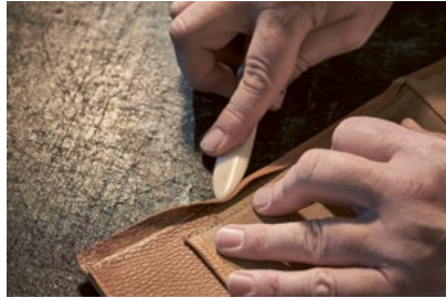
The edges of the individual parts of the bag are folded in using a folding bone.
