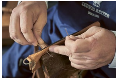
The handle and the side pleats are hand-stitched on the so-called "horse."
